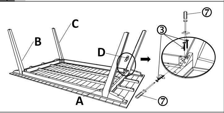
Attach the Wooden pad (D) to the table by using Short Screws (3) and Screw driver (7) as shown in picture below.
