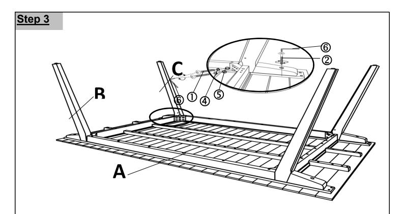
Attach Second Leg (C) to Table Top (A) as shown in picture above.
