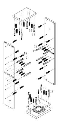
STEP 5 -Attach Top Board (1) & Bottom Board (4) onto Panel (2) & Panel (3)
