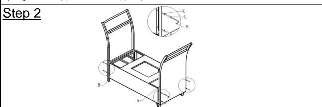
Attach Back Panel With Legs(B) to Bottom Basket(C) using Washers(K) and Bolts(L) with Allen Key(M) as shown in the picture.
