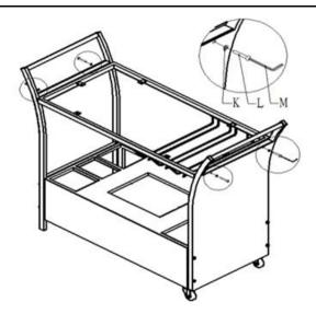
Attach Top Shelf Frame(D) between Back Panel With Legs(B) and Front Panel(A) using Washers(K) and Bolts(L) with Allen Key(M) as pictured above.
