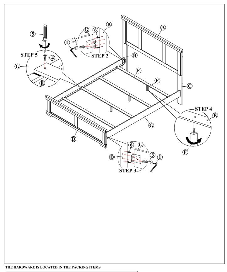
NOTE : MUST TIGHTEN SCREWS PERIODICALLY. WITH USE SCREW MAY BECOME LOOSE. CHECK TIGHNESS OF ALL SCREW EVERY 6-8 WEEKS.
