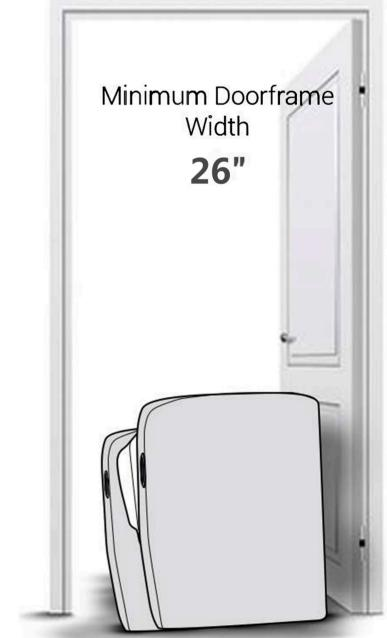
\*Rotate Chair 90° to fit through the door before attaching backrest
