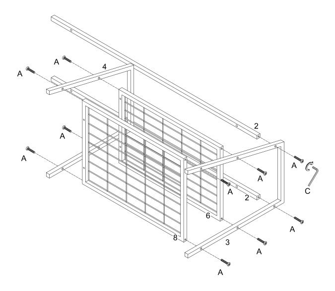
Using bolt (A) to secure parts (3, 4) to parts (2, 6, 8) with hex key (C) as per diagram.
