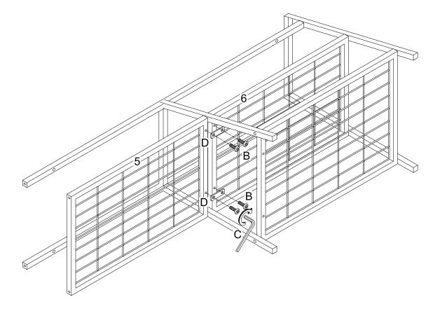
Using bolt (B) to secure part (5) to part (6) with hex key (C) as per diagram.
