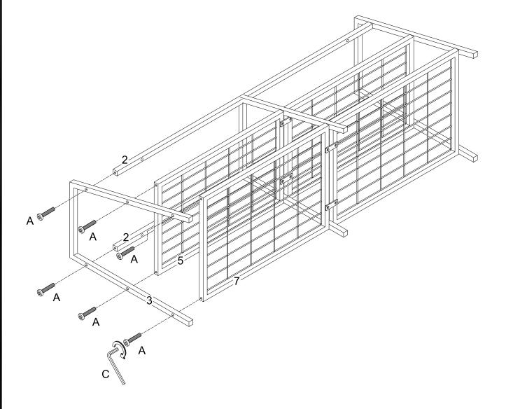
Using bolt (A) to secure part (3) to parts (2, 5, 7) with hex key (C) as per diagram.
