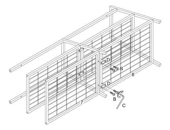
Using bolt (B) to secure part (7) to part (8) with hex key (C) as per diagram.
