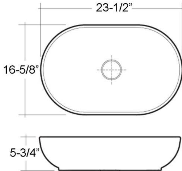
Dimensions of fixture are nominal and may vary within the range of tolerances established by AMSE Standard A112.19.2.2013 Dimensions and specifications subject to change without notice.
