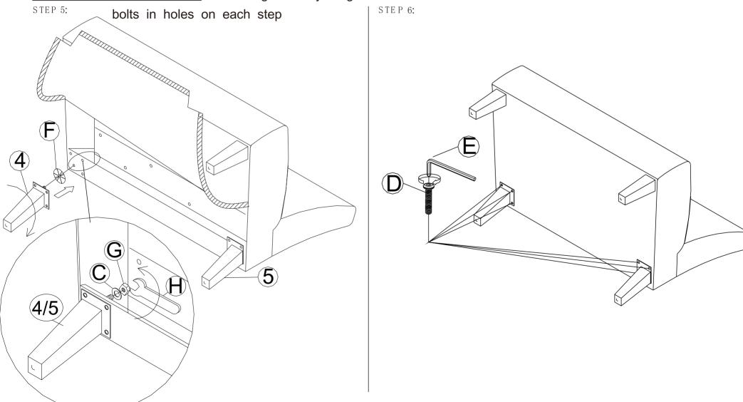
Assembly Instruction Please read and understand all assembly instructions before beginning assembly process. Do not tighten any single bolt until all bolts in holes on each step
