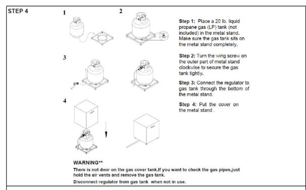
Place the 20lbs Propane Gas Tank (not included) into the Tank cover (09).
