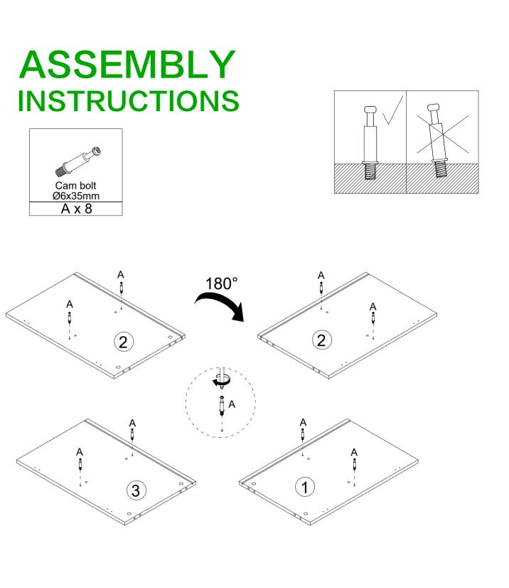
STEP 1 Insert cam bolts A into the settled holes on panels (123).
