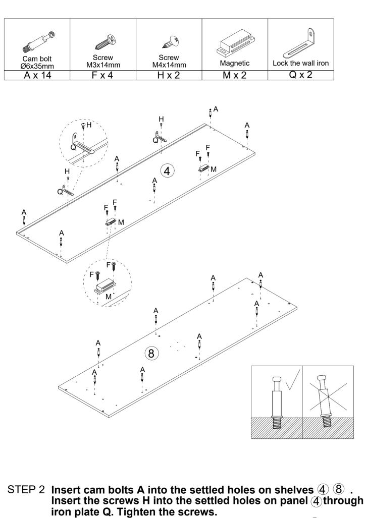
Insert the screws H into the settled holes on panel (4) through magnetics M. Tighten the screws.
