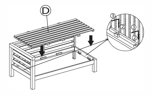
Attach the Seat Panel (D) into the Left Chair as shown in picture above. Affix Seat Panel (D) with Left Chair by using Screws (2) and Allen Key (3). Note: Using Screws (2) from inside to outside of Seat Panel (D)
