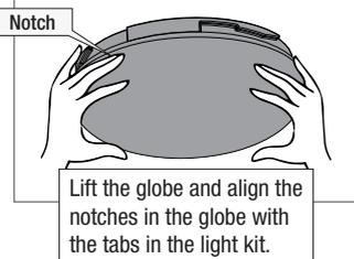
Lift the globe and align the notches in the globe with the tabs in the light kit.
