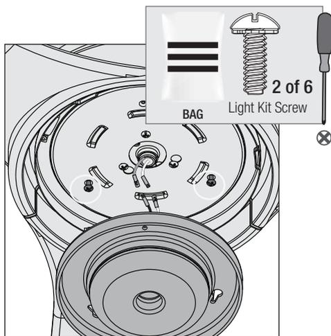
Partially install two of the light kit screws found in the hardware bag. It does not matter which two screw holes you choose. Connect the single-pin connectors from the LED assembly to the connectors from the fan. Connect the white wires together. Connect the blue and black wires together.
