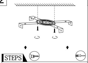
Lift the ceiling plate of the whole lamp to the hole of the hanging plate, and fix it with screws
