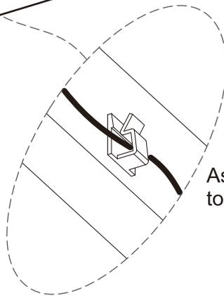
As required, add or remove accessory **K** (
