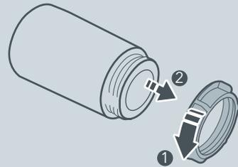
Loosen the red lock nut on the extension column in anticlockwise direction.
