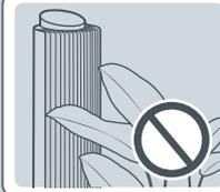
**DO NOT** block or cover air flow to or from the fan while in operation.
