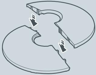
Connect the front and rear base parts by pushing the plastic pegs on one half into the corresponding slots on the other half.
