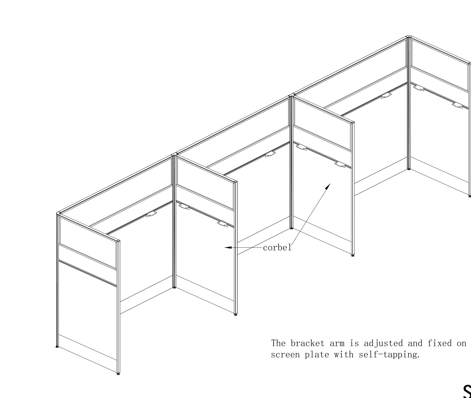
The bracket arm is adjusted and fixed on the
