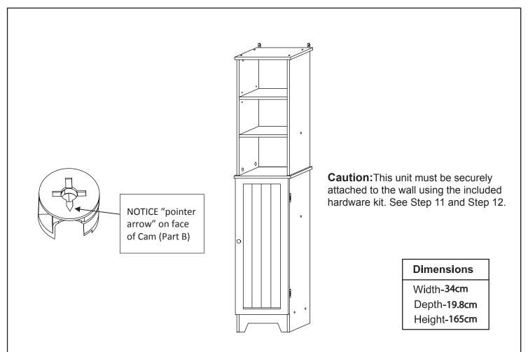
Place the Cam so that the "pointer arrow" faces the edge of the panel. This allows for the Pin (Part B) to be correctly aligned with the opening of the Cam.
