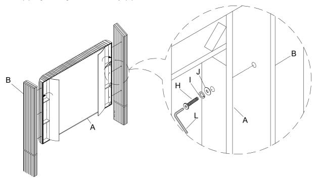
2 Attach Rectangle Plate (M) to the Side Rail (D) and H/B Poster (L & R) (B) by using Allen Bolt (G), Spring Washer (I) and Flat Washer (J). Unfasten bolts on Footboard (C), then attach Side Rail (D) to Footboard (C) and tighten all bolts with Allen Key (L).
