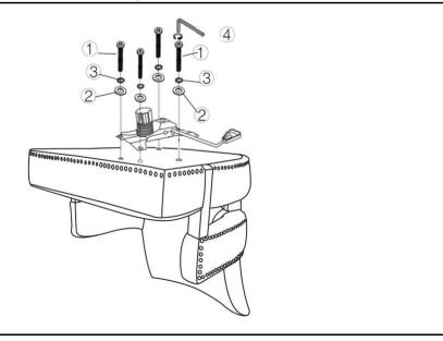
Attach Mechanism(B) to Chair Seat(A) using Bolts(1), Washers(2), and Spring Washers(3) with Allen Key(4).
