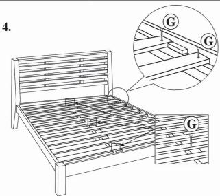
Lay the slats (P7) between the side rail (P3) using hardware:
