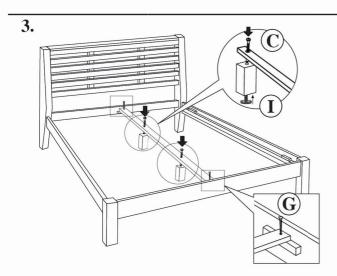
Fix the adjuster (I) to the support leg (P6) using hardware:
