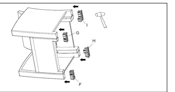
Attach the Left Front Foot Clip(F), Right Front Foot Clip(G), Left Back Foot Clip(H), Right Back Foot Clip(I) to the feet of the Club Chair using the Rubber Hammer(Q) as shown above.
