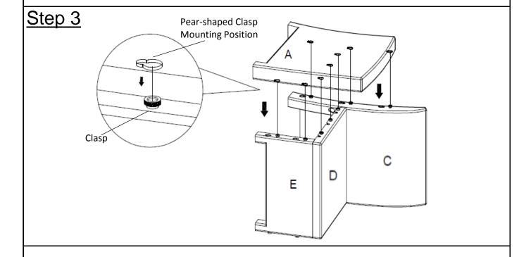
Turn the assembly onto it's side as shown.
