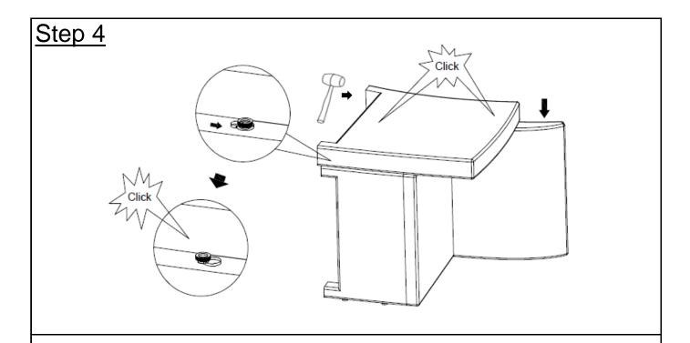
Button up the Clasps with the Rubber Hammer(Q) from left to right as shown above.
