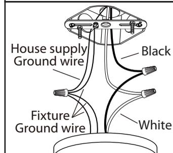
3. Connect the ground wires (bare copper or green) from your fixture to the ground wire (bare copper or green) or ground screw in the electrical box. Connect the black wire from the fixture to the black wire in the electrical box and connect the white wire from the fixture to the white wire in the electrical box.
