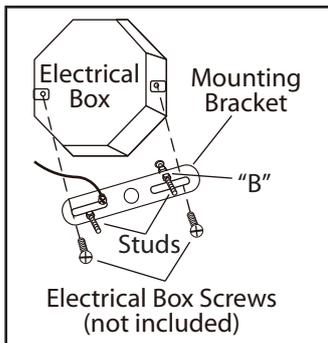
**Note:** Determine desired mounting option prior to proceeding with installation.
