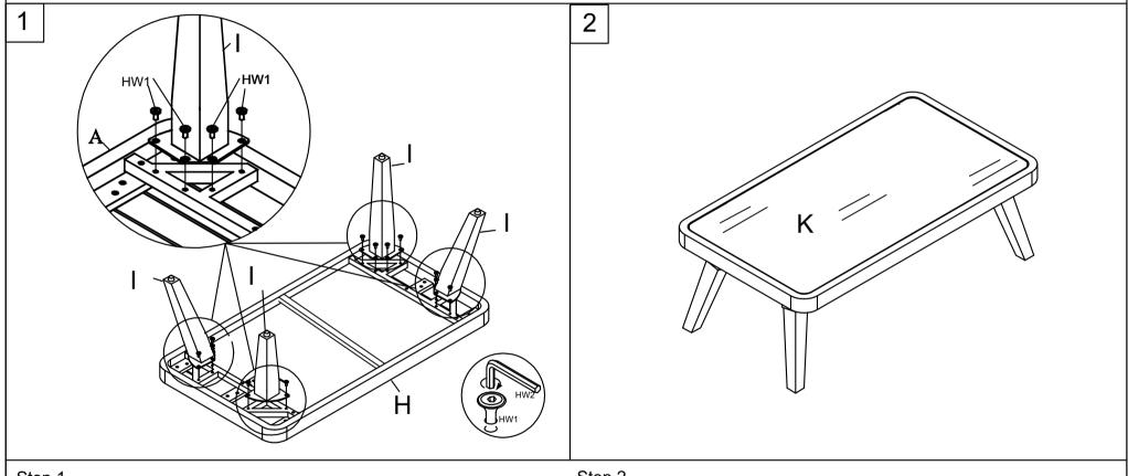
Step 1 Attach Leg (I) to Table Top (H). Use Bolt (HW1) tighten with Allen Key (HW2).
