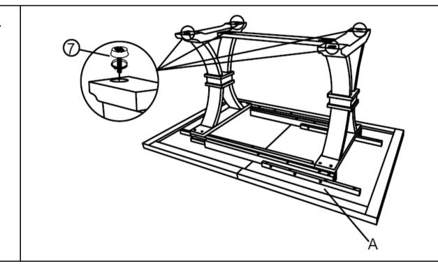
Insert the Adjustable Gliders (7) into the Table Base (B) as shown above. **FULLY TIGHTHEN ALL THE BOLTS.**
