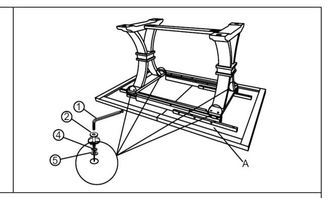
Place the Table Top (A) on a clean, non-marring surface, then place the assembled table parts from Step 3 on top of it. Affix the Table Top (A) to the Table Base (B) with Bolts (2), Spring Washer Rings (4) & Flat Washer Rings (5) using the Allen Wrench (1).
