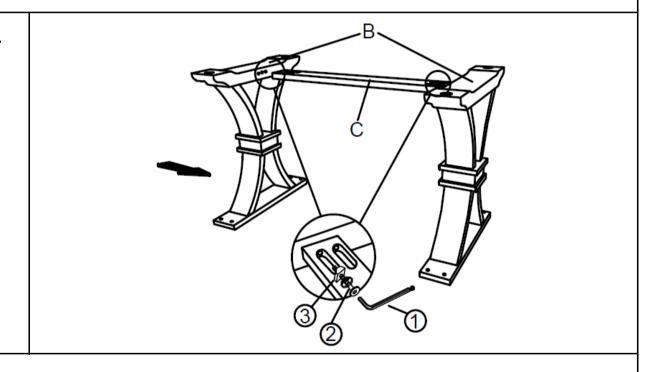
Attach the Crossbar (C) to the Table Base (B) using Bolts (2), Crescent Nuts (3) and the Allen Wrench (1).
