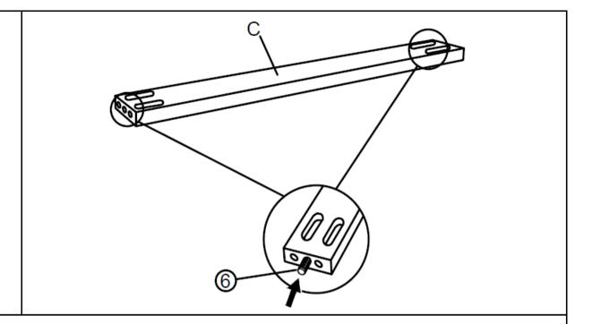
Insert PVC Dowels (6) into the Crossbar (C) as shown above.
