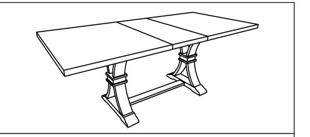
Place the Table on a LEVEL SURFACE and check that it is balanced. If there is a slight wobble, please adjust the Adjustable Gliders (7). EXERT pressure floorwards, onto the Table.
