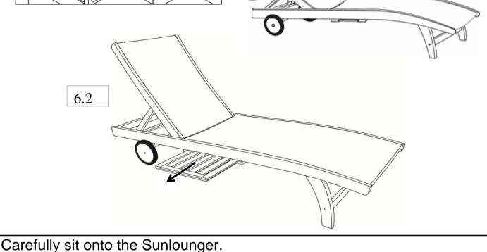
This pressure will help the Sunlounger reach full alignment at all joints. In a sequential manner, gradually tighten all Bolts and Screws until evenly secured.
