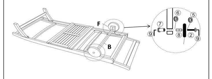
Attach one of Wheel (F) to Back Leg Panel (B) by using Bolt (2), Washer (5), Iron tube for Wheel (8), Washer (6) and Sleeve Nut (7) with Allen Key (9) in sequence as shown on the picture above.
