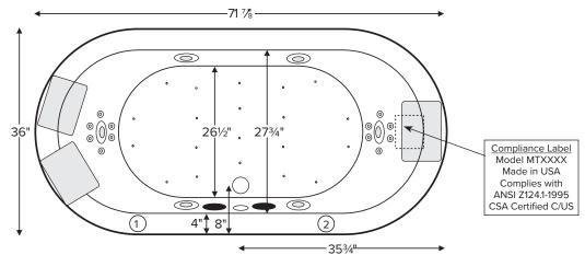
Numbered areas on tub deck represent possible locations to install cleaning systems, faucets and other fixtures. When Fill-Flush is ordered and location 2 is chosen, the detergent feeder will need to be offset to the left or the right. Shown with Air Massage and Ultra Whirlpool Package.
