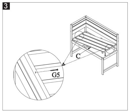
Step 3: put the seat (C) to the bench as shown on the picture. Then use the screw (G5) to tighten the seat (C) to the bench.
