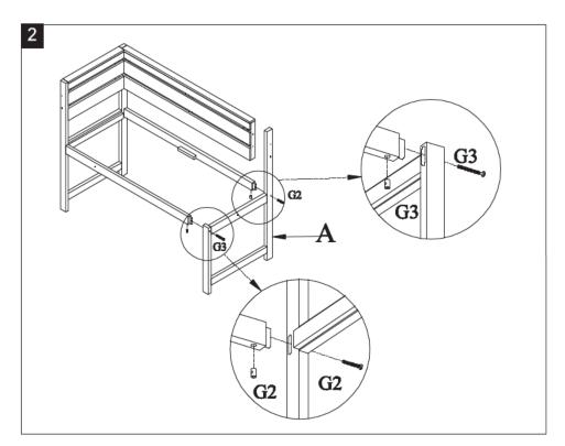
Step 2: attach the leg(A) to the back (D),rear bar (E) and front bar (F) as shown on the picture. Then use the Allen bolt S (G2) to tighten the leg (A) to the rear bar (E). Use the Allen bolt L (G3) to tighten the leg to the front bar (F) as shown on the picture.
