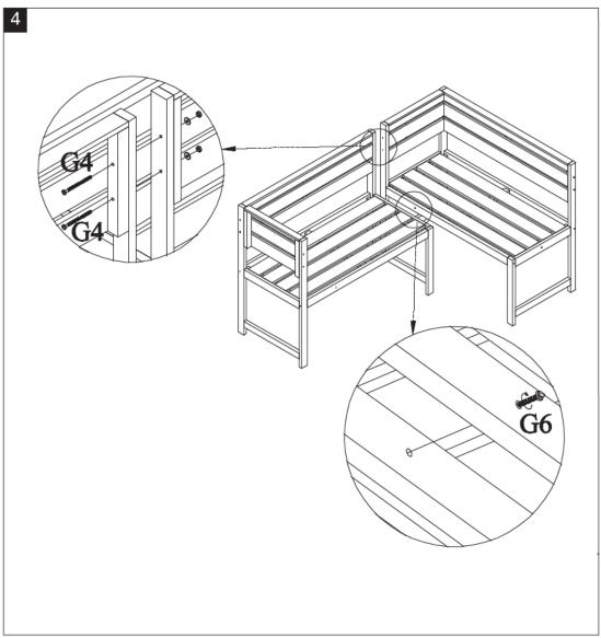
Step4: repeat same step with other bench and connect 2 benches together as shown on the picture. Then use the Allen nut L (G4) to tighten the back together as shown on the picture. Lock 2 benches by turn on the bolt under seat to the hole as shown on the picture.
