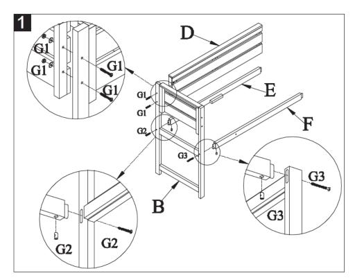
Step 1 : attach the side (B) to the back (D),rear bar (E) and front bar (F) as shown on the picture. Then use the Allen nut S (G1) and the Allen bolt S (G2) to tighten the side (B) to the back (D) and rear bar (E) . Use the Allen bolt L (G3) to tighten the side the front bar (F) as shown on the picture.
