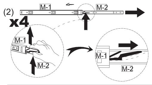
Move the black paddle upward and pull out (M-2) to the right.
