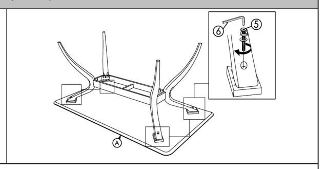
Place the Table top (A) on a soft surface to avoid any scratches or damages to the product and place the Table Leg with the table supporter onto the of table top support with your adult partner.
