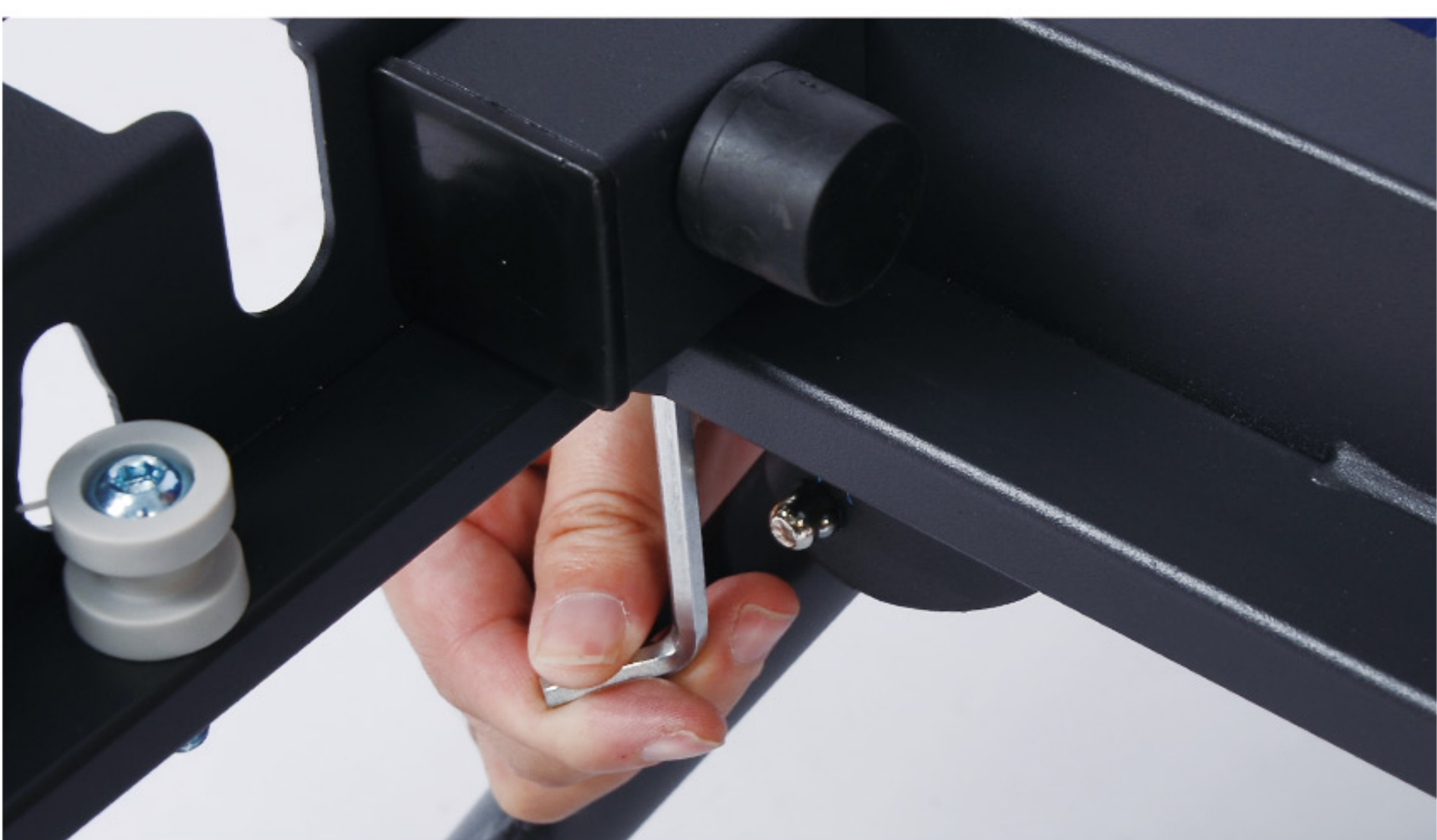
22. Use a hex wrench to tighten the bolts.
