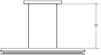
(1) Measure the desired height (H) of the fixture.
