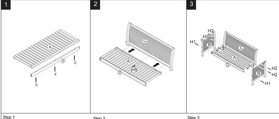
Attach seat frame (A) to cross bar of leg (D), use screws (E) and tighten with allen key (H4).
