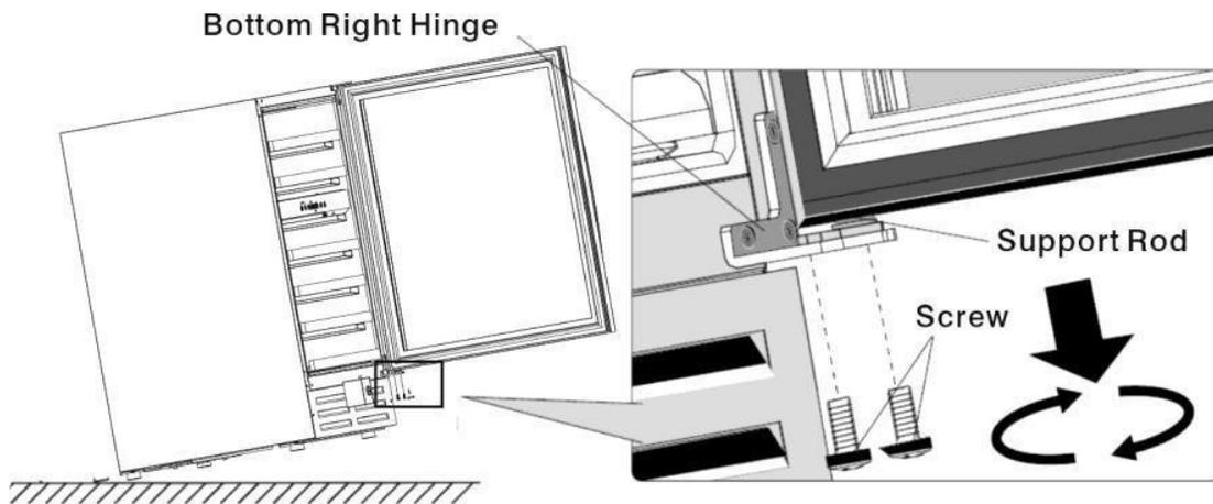
2. Remove the door off the upper hinge and take out the support rod.
