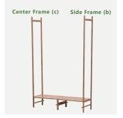
4 Connect Center Frame (c) and Side Frame (b) with the completed Stand as picture shown. Secure them with Medium Screws (s).
