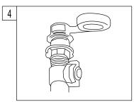
Thread mounting nut and bottom gasket onto drain body. Wrap top threaded end of the drain body with plumbers' tape.
