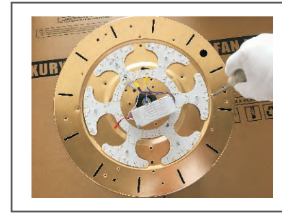
Step 4. Remove the main engine chassis screws.
