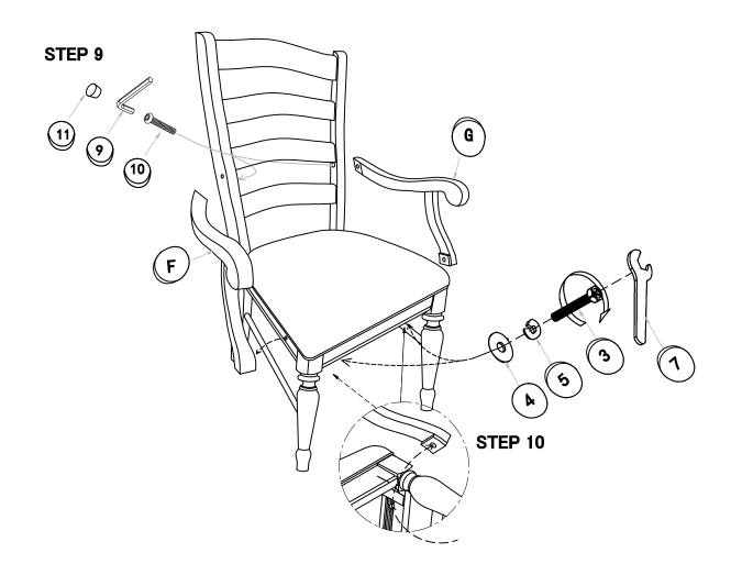
\* Turn the chair to the standing position. Check its balance and tighten all screw and bolts to complete the assembly.
