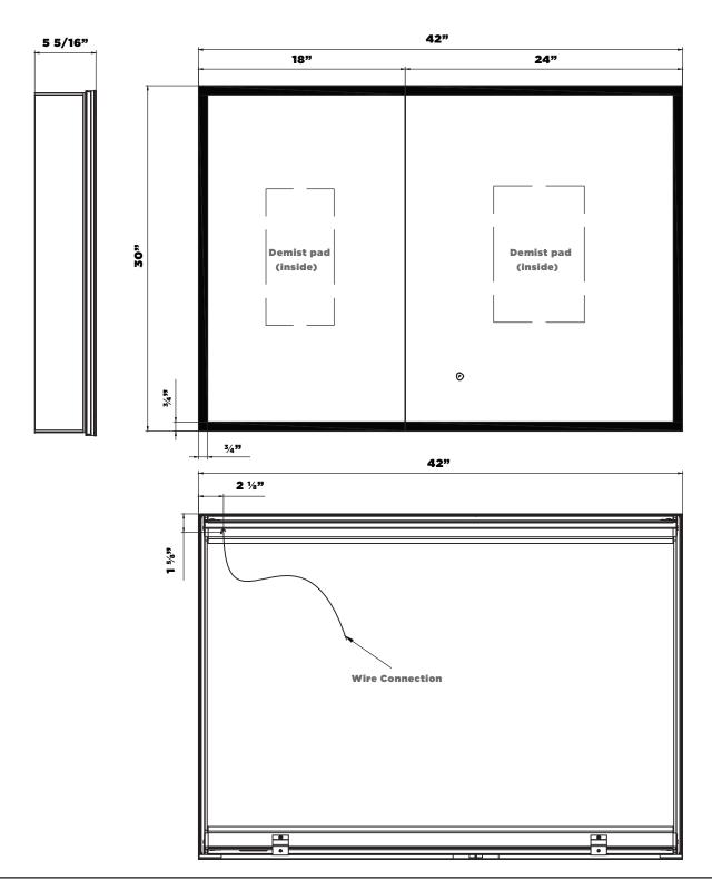
**ATTENTION!** Dimensions may vary by up to 3/8". It is highly recommended to pull all dimensions of actual model for installation and measuring purposes.
