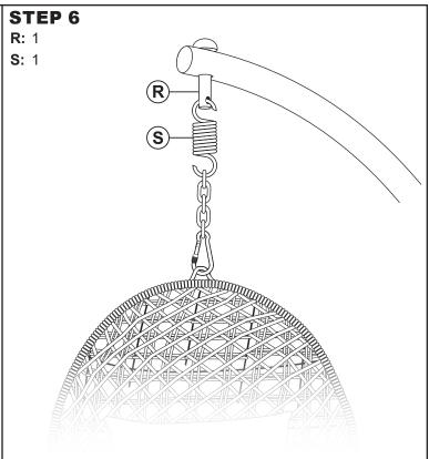
Place Pin (R) into the top of the curved pole. Insert Extension Spring (S) through the bottom of Pin (R).
