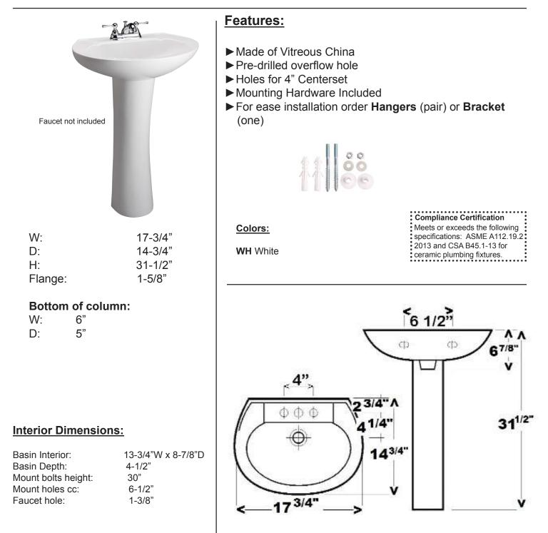
Dimensions of fixture are nominal and may vary within the range of tolerances established by ANSI Standard A112.19.2-2013. Dimensions and specifications subject to change without notice.
