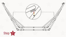
Attach the short diagonal bar to the chosen notch on the main diagonal bar by threading the bolt onto the notch. Push down until a click sound is clearly heard.
