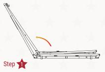
Put the base stand horizontally on your chosen surface. Extend the main diagonal bar.
