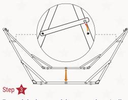
Expand the hammock base stand vertically. Connect the cross bar to the notch on the opposite main bar.
