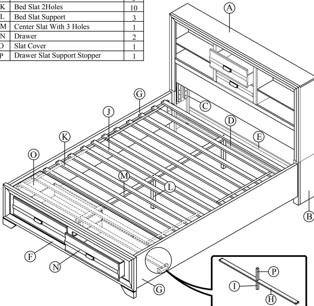
STEP 1.1: Attach & tighten the Headboard Leg (B) & (C) to the Headboard (A). Affix Headboard & Headboard Leg using JCBC screw M6 x 35mm (4), Spring Washer (6), Flat Washer (7) using L Key (8).
