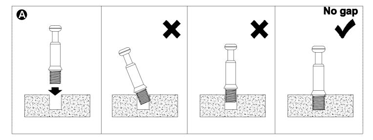
Screw the pin into the hole. Set the cams correctly by aligning the head of the cams with the lock pins. Lock the cam by turning the cam head with a screwdriver until it is tightened. Please do not use an electric screwdriver to assemble the unit.
