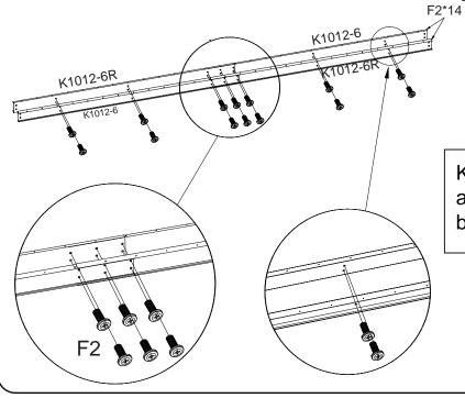
K1012-6 is smaller in width and fits into the K1012-6R bore for alignment.
