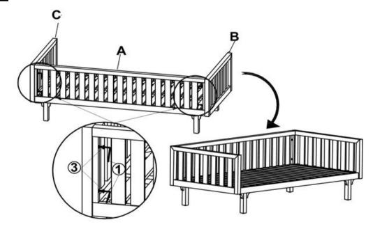
With assistance from your adult partners, stand the assembled parts in step 4 up. Attach the Backrest Panel (A) to the Left Panel (B) and the Right Panel (C) by using 4 Botls (3) with Allen Wrench (1).
