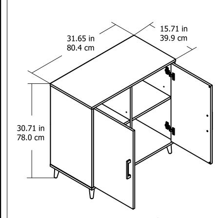
Door Area dimensions: 29.52 in. (75.0 cm) W 25.11 in. (63.8 cm) H 14.72 in. (37.4 cm) D 1.58 cubic feet each storage area
