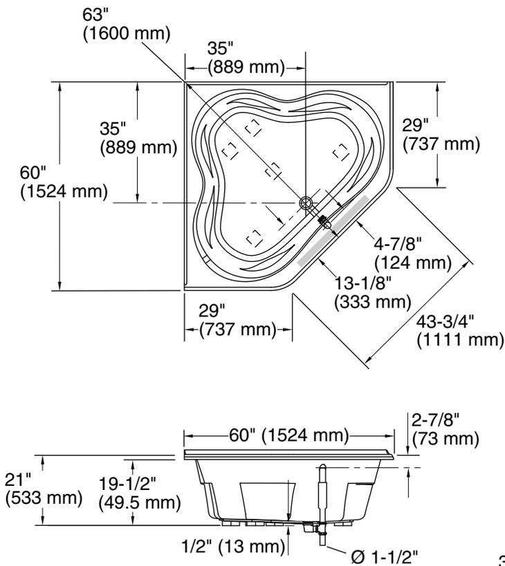
No change in measurements if connected with drain illustrated. (K-11677 or K-11677M)
