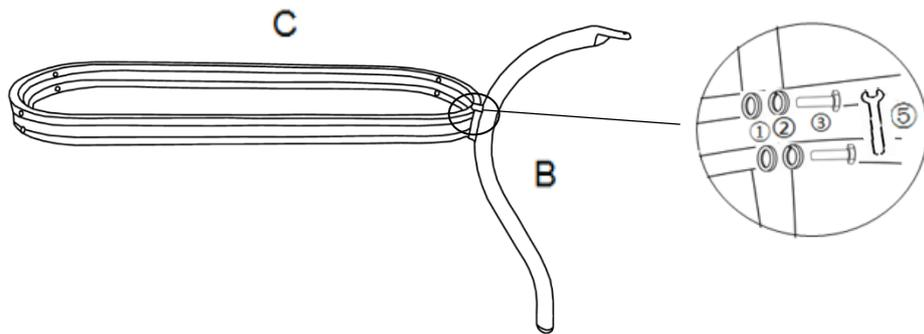
Loosely attach the Central Support Ring(C) to Table Legs(B) using washers(①), Spring Washer(②), and Hex Bolts(③), with the Spanner(⑤).
