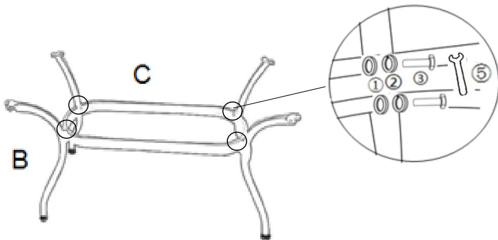
Repeat step 2, attaching the remaining 3 legs to the Central Support Ring(C)
