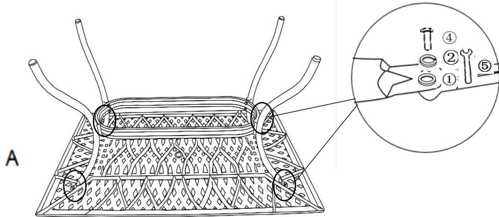
Lay the Table Top(A), top facedown, onto a flat, soft, clean surface. Attach the Table Legs(B) to the Table Top(A) using Washers(①), Spring Washers(②) and Hex Bolt (④) with the Spanner(⑤).
