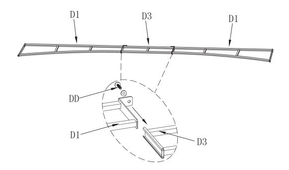
Please find 2 PCS of D1 and assemble them into each end of D3 by using Screws DD.
