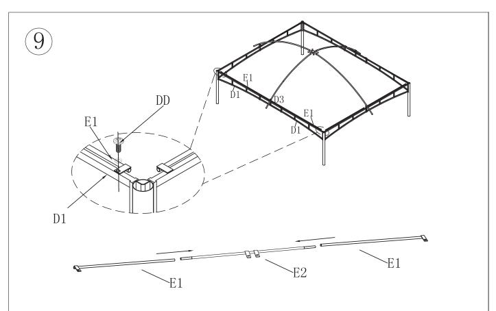
Please also connect each end (E1) of Slider to D1 by using Screws DD.
