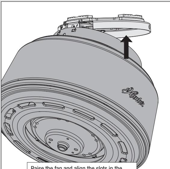
Raise the fan and align the slots in the canopy with the hooks on the ceiling plate.
