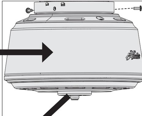
Hold the canopy up with the screw holes aligned. Partially install two canopy screws, found in the ● hardware bag, into the holes opposite the ceiling plate hooks.
