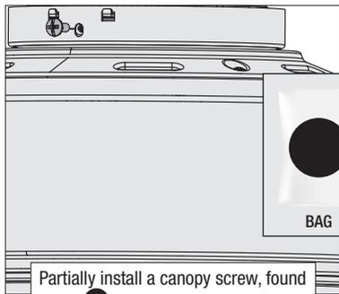
Partially install a canopy screw, found in the ● hardware bag, between the ceiling plate hooks. When all the holes are properly aligned, securely tighten all three canopy screws.
