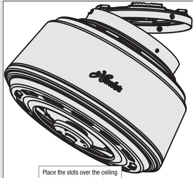
Place the slots over the ceiling plate hooks to hang the fan.
